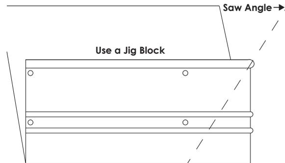
The finish opening must be square for the proper finished miters on the cladding. Lay out all parts to make sure you do not use the header for one of the verticals.
